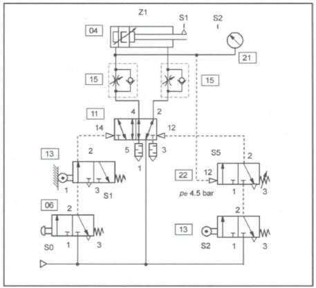
Figure 2.6: Pressure dependent control of a double-acting cylinder
