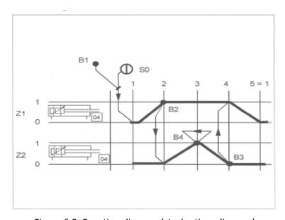
Figure 6.2: Function diagram (stroke-time diagram)
