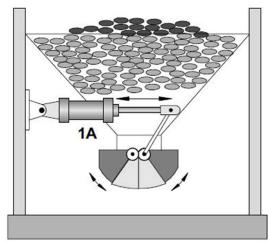
Fig. 3.4 Positional sketch of the hopper machine
