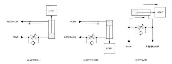
Fig.4 Basic flow control circuits
