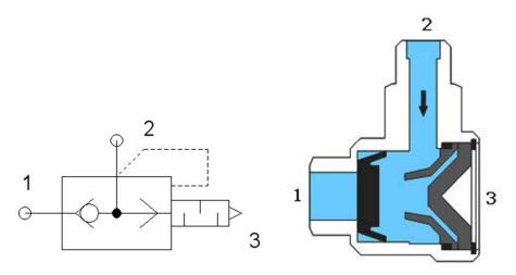
Fig. 5.2. ISO symbol of quick exhaust valve
