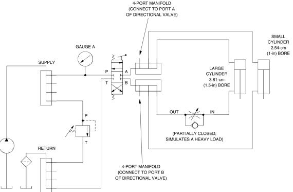
Fig.3. Cylinders in parallel with a heavy load on the large cylinder
