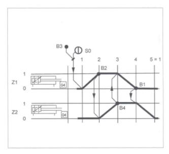
Figure 6.1: Function diagram (stroke-time diagram)
