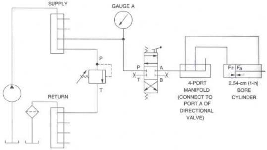
Fig. 9 Schematic diagram of Applying equal pressure on both sides of a piston.
