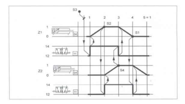
Fig.5.7 Function diagram (stroke-time diagram)
