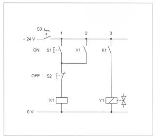
Figure 3.8: Electric circuit diagram (dominant "off")
