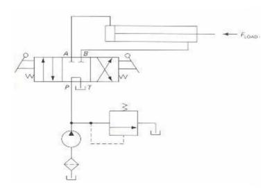
Fig.1 Double Acting Cylinder Control Circuit
