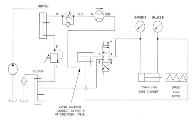
Fig.1 Cylinder in a regenerative circuit.
