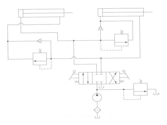
Fig.1 Hydraulic Sequence Circuit
