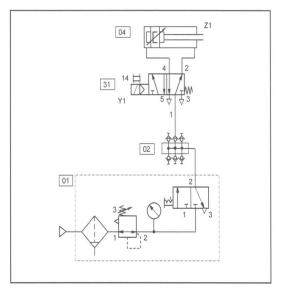
Figure 3.7: Pneumatic circuit diagram
