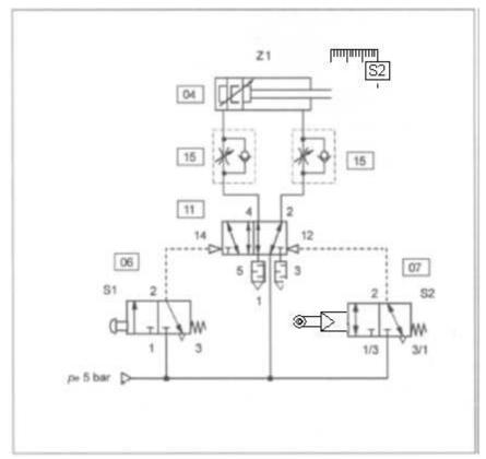
Figure 2.4: Controlling a double-acting cylinder by impulse valve
