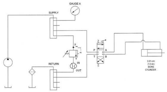
Fig. 2 Schematic diagram of the cylinder actuation circuit
