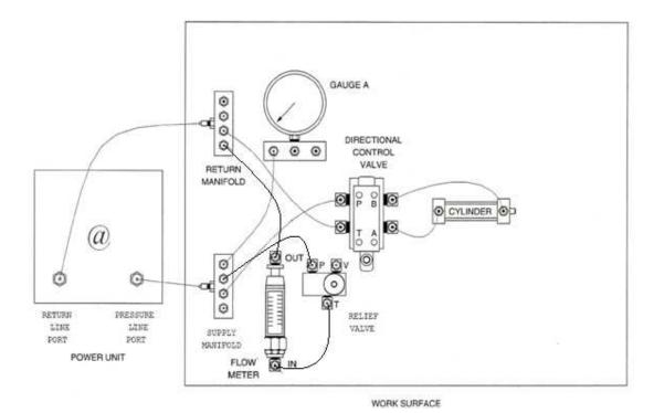
Fig.3 Connection diagram of the cylinder actuation circuit
