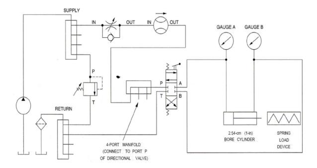
Fig.2 Cylinder in a normal (non regenerative circuit).
