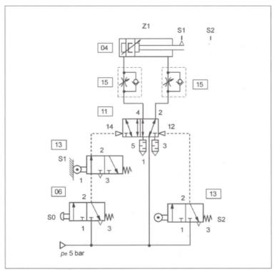
Figure 2.4: Displacement dependent control of a double-acting cylinder
