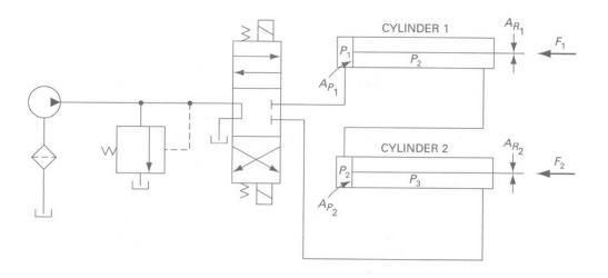
Fig.3 Series Cylinder Circuit
