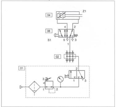
Figure 2.1: Direct control of a double-acting cylinder
