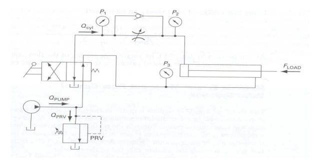
Fig.3 Meter-in speed control of hydraulic cylinder during extending stroke
