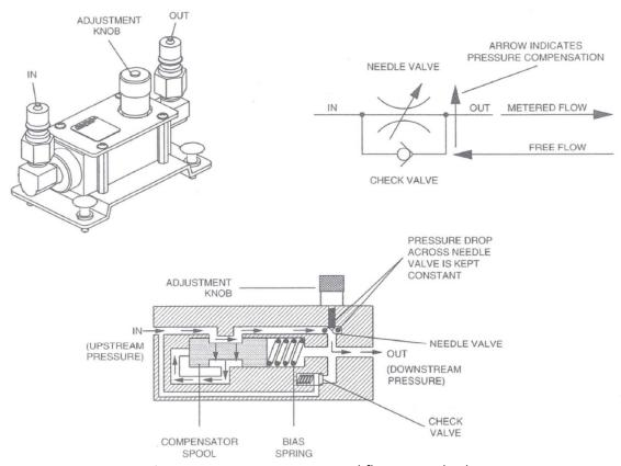
Figure 1, Pressure compensated flow control valve
