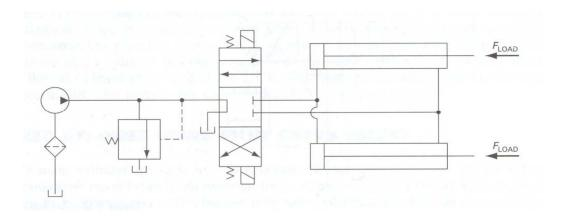
Fig.2 Parallel Cylinder Circuit
