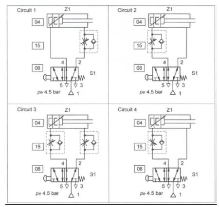
Figure 2.2: Speed regulation of a double-acting cylinder
